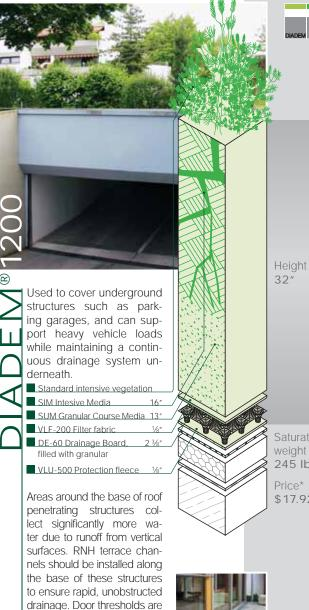
made from 100% pre-consumer recycled polystyrene. Each 3 ft×6 ft board is double-formed on both sides with interlocking cups to passively distribute water over the entire surface area. This increases retention capacity and increases irrigation efficiency. For inverted roofs, boards help
